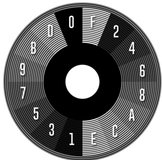
Figure 4. Interleaved Z-Code
